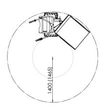
All dimensions unless otherwise stated are in millimetres. Dimensions TB300 BENDI (TB450 BENDI)
