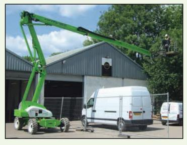
The HR21 Hybrid AWD also incorporates **ToughCage** and **SiOPS®** technologies. A tough impact resistant composite base and larger cross-section steel give the ToughCage strength and durability, while SiOPS® offers additional operator protection.
