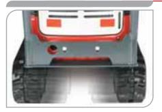
**EXPANDABLE TRACK FRAME** The TB108 has a unique expanding track frame to adjust from 680mm to 900mm allowing it to travel through narrow openings. Added track width then gives greater operating stability.
